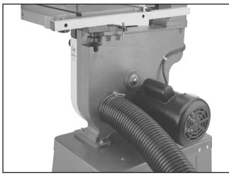
Figure 25. 4" dust hose attached to dust port.
